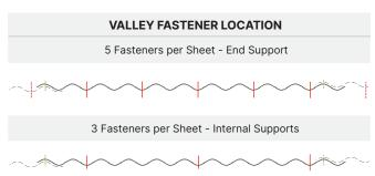
NOTE: Side lap fasteners are optional when using 5 fasteners per sheet, but are a requirement when only using 3 fasteners per sheet for valleys.
